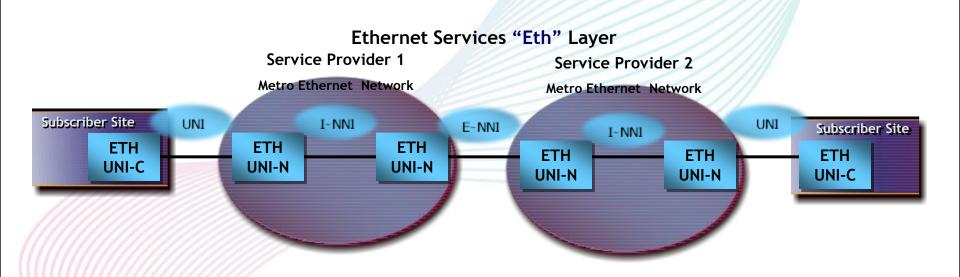
UNI: User Network Interface, UNI-C: UNI-customer side, UNI-N network side NNI: Network to Network Interface, E-NNI: External NNI; I-NNI Internal NNI
