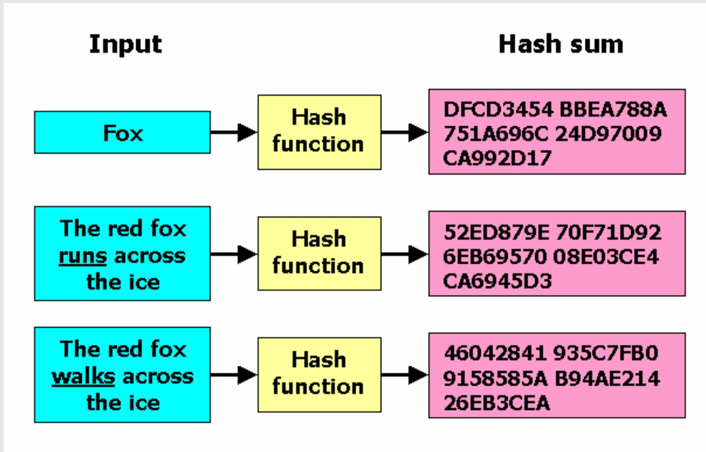
Note the significant change in the hash sum for minor changes in the input. Note that the hash sum is the same length for varying input sizes. This is extremely useful.
