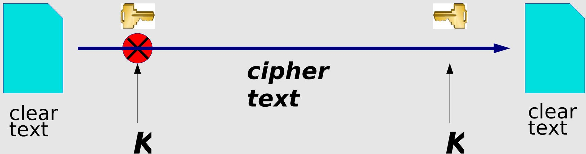
The same key is used to encrypt the document before sending and to decrypt it once it is received
