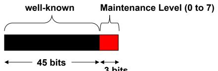
Transmitted at a configurable periodic interval by MEPs (default is 30 seconds, range from 10 sec to 65535 sec.)
