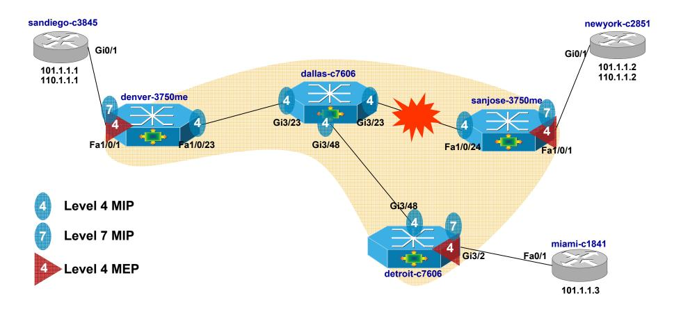
SNMP Traps are generated when a remote MEP is not heard from.
