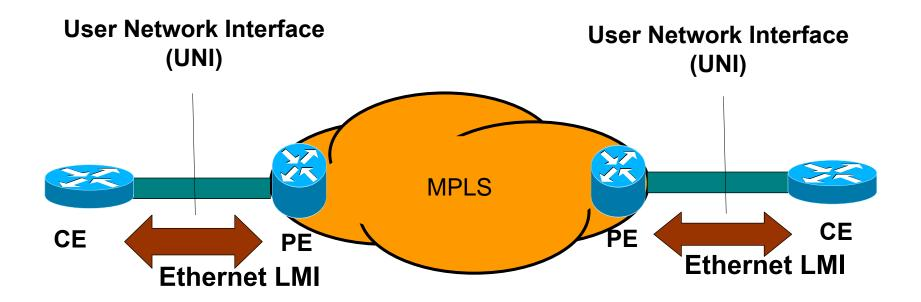
Ethernet LMI: Ethernet Provisioning and Management entity across UNI (CE-PE)
