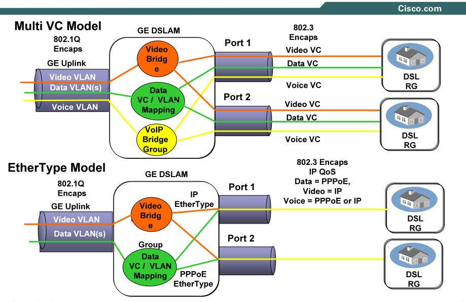
**Layer 2 RG Physical Port Based Service Mapping**
