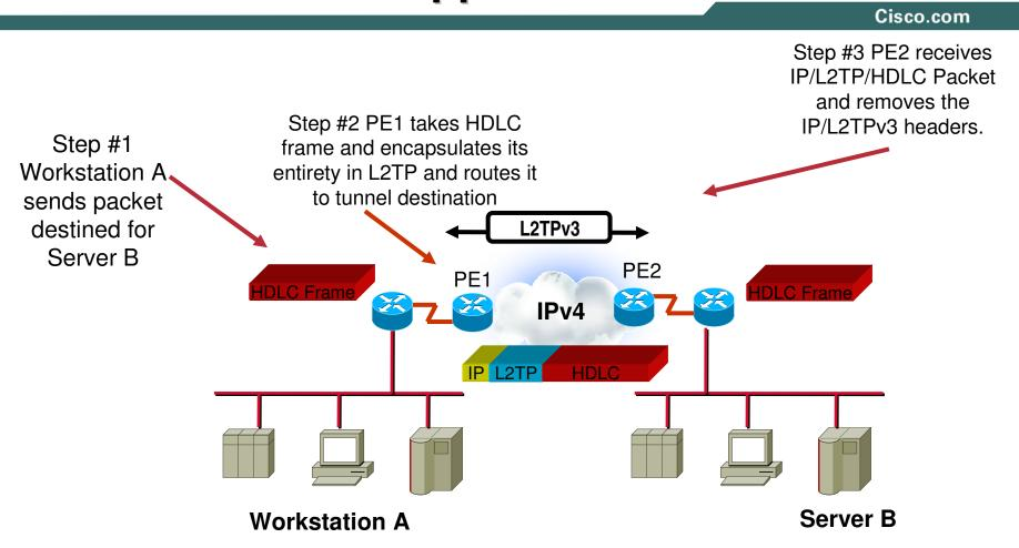
A portion of an HDLC or PPP leased line is emulated over an IP network. To the end user devices, the leased line appears as a single segment.
