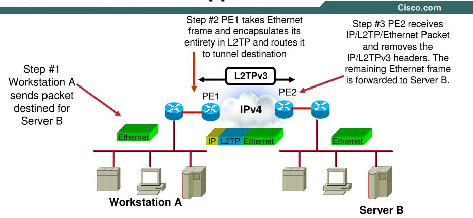
Two Ethernet Segments are joined over an IP core via L2TPv3. To the end user devices, the two physical Ethernet networks appear as a single segment.
