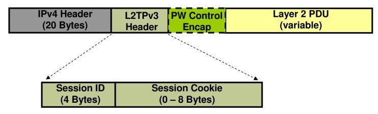
IPv4 Header - The delivery header for the Tunnel. Always destined for an LCCE.
