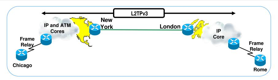
**Requirement:** Frame Relay connections between Chicago & Rome
